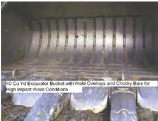
40 Cu Yd Excavator Bucket with Weld Overlays and Chocky Bars for High Impact Wear Conditions
